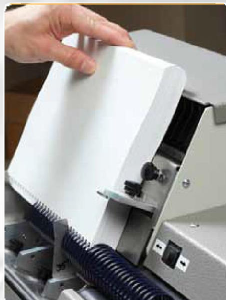
Book shaping spine formers enable the operator to insert diameters up to 50 mm.
